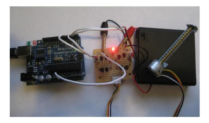
Arduino Stepper Motor Serial Control Cable
